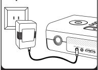
jack on back of the iP99 and plug the other end into a working wall socket.
